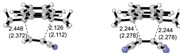
Figure 6. MPW1K optimized geometries of the transition structures of the Diels–Alder reactions of 9,10-dimethylantracene with cyanoethylene and tetracyanoethylene (values in brackets are for HF/6-31G*).
